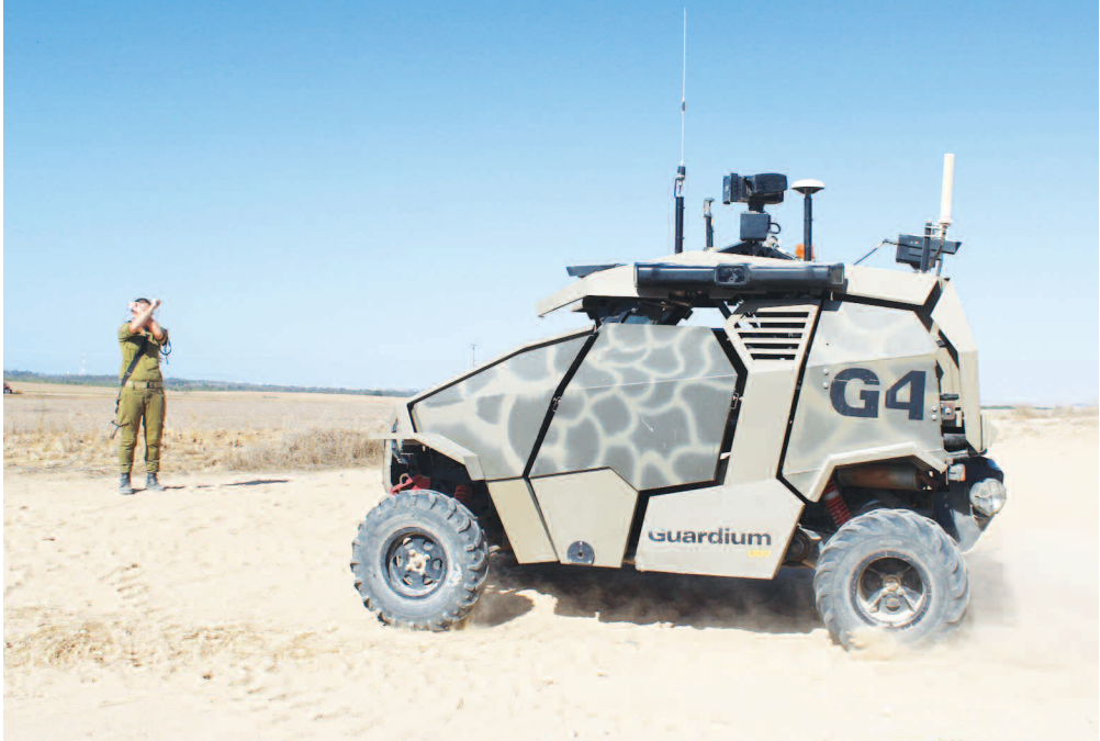
IAI Lahav's Gurdium, a UGV based on a lightweight Tomcar chassis that went into service with the Israel Defence Force (IDF) as a border patrol asset in 2009
