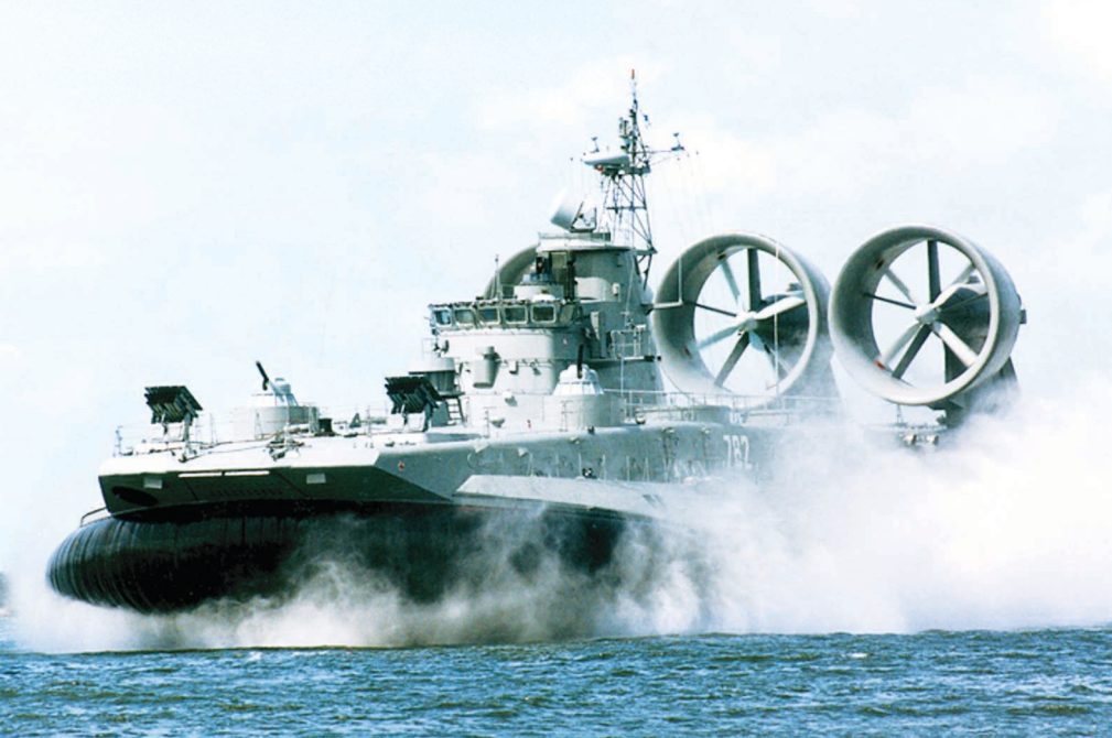
The Russian military with the 555 tonne Almaz Project 12322 Zubr, has the distinction of operating the largest and most heavily armed hovercraft in the world
