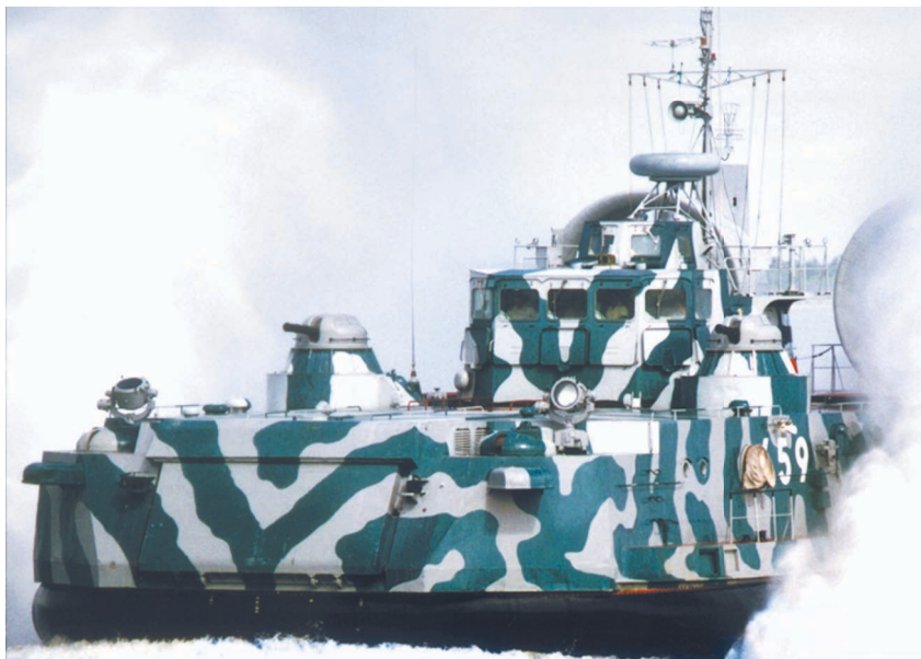
Almaz also offers the 150 tonne Project 12061 Murena-E (Moray) aluminium-magnesium hovercraft, which is also primarily intended as an amphibious assault vehicle with fire support and mine laying capabilities
