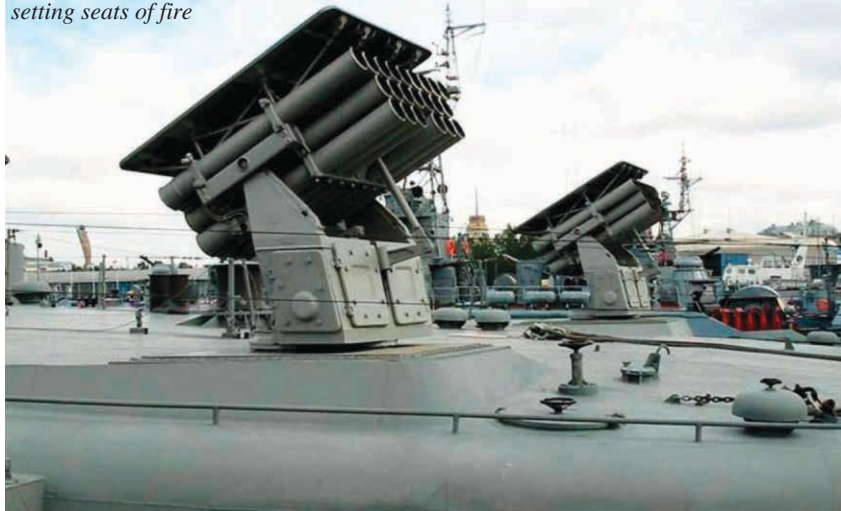
The A-22 Ogon MRL system is intended to equip the river and landing ships, including hovercraft, and provides: engagement of the area targets on the shore, equipment and manpower in the coastal zone, surface targets (boats, waterborne platforms), and setting seats of fire
