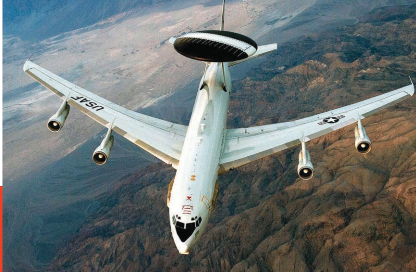
The 707 aircraft a prime example in both E-3 Sentry AEW&C and E-8 Joint Surveillance and Target Acquisition Radar System (JSTARS) form, as well as many EW and command and control variants. Photo : Boeing
