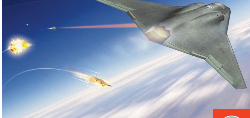
Northrop Grumman's 6th generation concept is also tailless, and this illustration shows that high energy lasers are under consideration for hard kill defence against advanced air-to-air missiles. Like the Boeing concept, it includes a pilot. (Northrop Grumman image)
