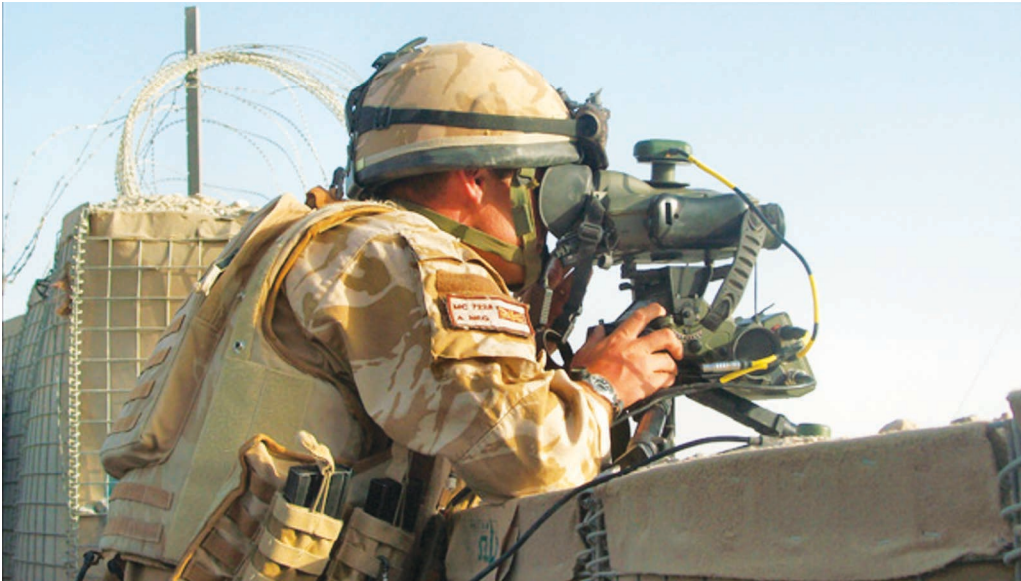
Rockwell Collins continues to promote FireStorm, a scalable and wearable targeting system designed to provide full digital interoperability with coalition aircraft and artillery systems
