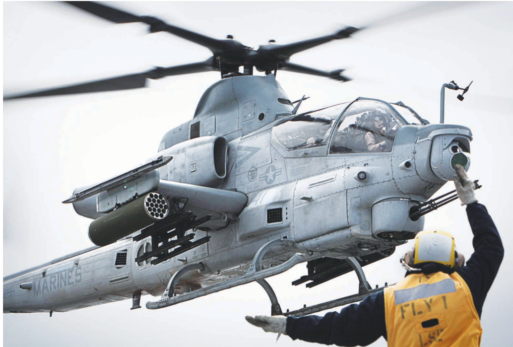
The AH-1Z Cobra attack helicopter's Lockheed Martin Target Sight System (TSS)
