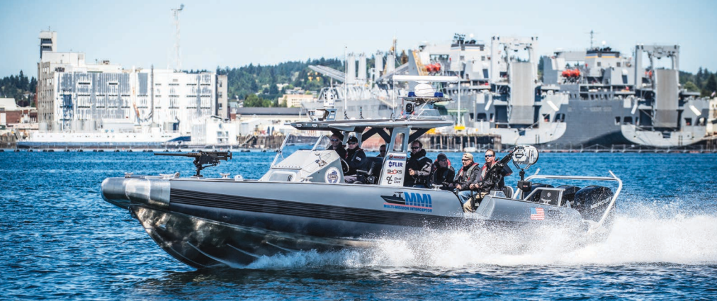
Cruising at 35kt, the MMI has a range of more than 200 nm, says the company, remains operational in sea states up to five and survivable up to six. The boat weighs 4,865 kg unladen and can carry loads of up to 2,704 kg consisting of fuel, people and cargo. Photo: SAFE Boats
