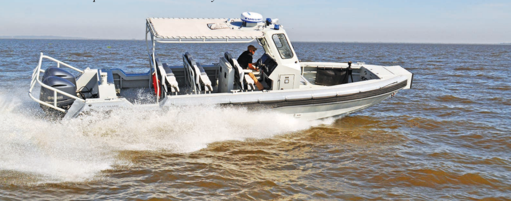
The 33 Relentless is a twin-engine, centre console design in aluminium by naval architect Michael Peters that has been chosen by many law enforcement and military operators. Photo: Rival yard Metal Shark
