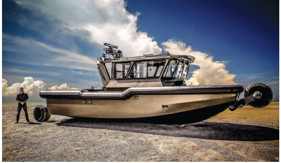
The amphibious mobility bestowed by Sealegs opens up many more potential launch and recovery locations, extends patrol capabilities into very shallow water and even allows the boat to take up an observation position on land if necessary.
