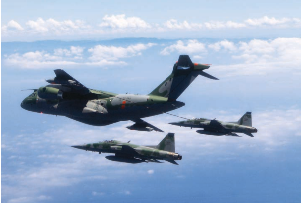
Embraer KC-390 tanker on an early AAR test with a pair of F5 fighters. This was a dry contact in which no fuel was delivered. Photo: Embraer
