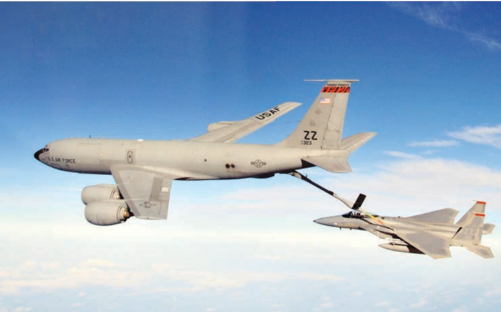
A KC-135R Stratotanker, the mainstay of the USAF's AAR fleet, refuels an F-15C Eagle
