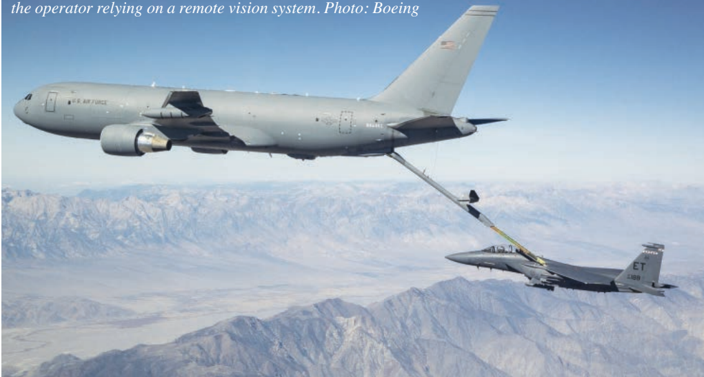
F-15 receives fuel via the boom of a Boeing KC-46. The boom is operated remotely from a position near the tanker's cockpit, the operator relying on a remote vision system. Photo: Boeing
