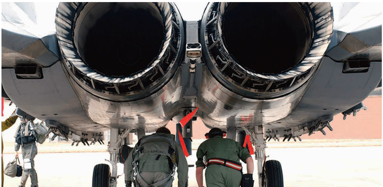
The propulsion system of F-15 consist of two F100-229 Engines
