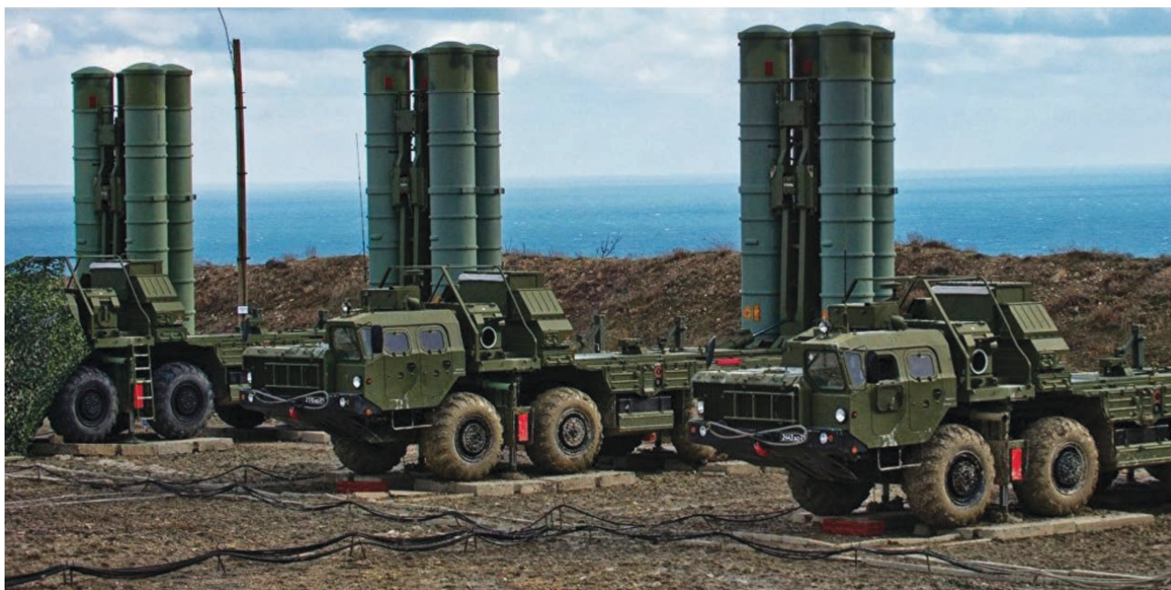
Missile tubes erected into vertical launch position. Cables link the TELs to the command post, enabling distributed deployment to reduce vulnerability to adversary defence suppression/destruction weapons. (Russian Defence Ministry)
