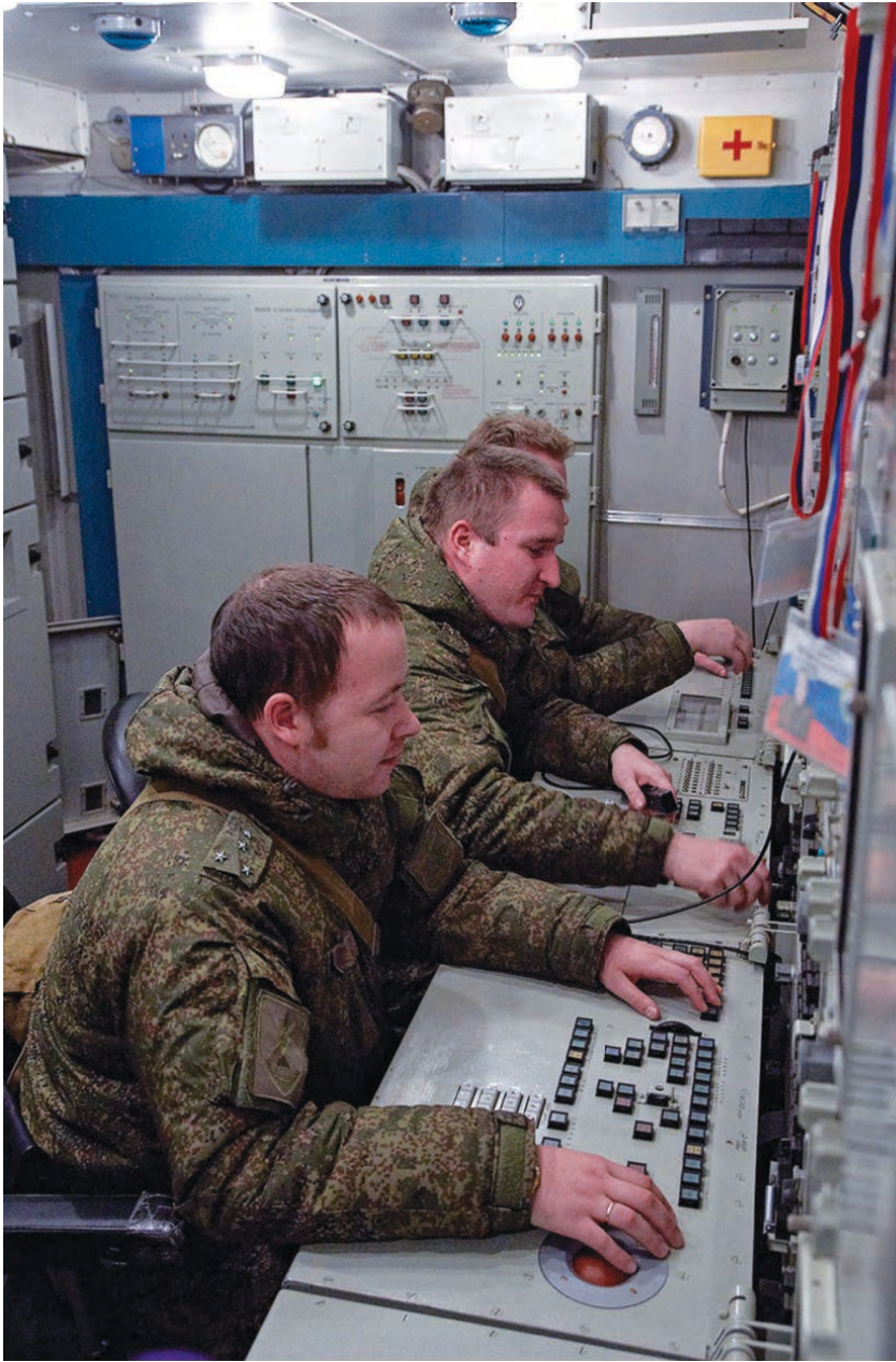
Integrated into a truck-mounted container, the 55K6E command post gathers information from and controls a group of missile batteries, and can also control the Big Bird radar via a command, control and communications data link system. (Russian Defence Ministry via Wikipedia)
