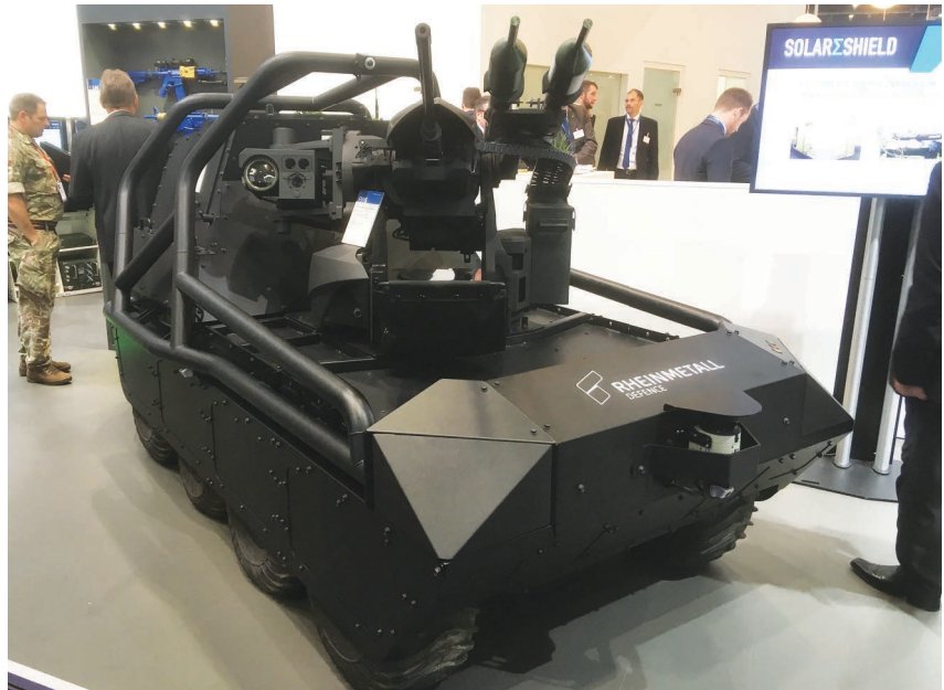
Rheinmetall outlined its Multi-Mission Unmanned Ground Vehicle (MMUGV) solution that is intended to enable the platform to carry out missions ranging from logistics mule duties to surveillance and force protection in support of mounted and dismounted forces in dangerous and hard to reach areas
