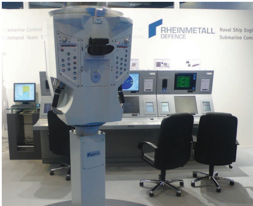
The Periscope Simulator (PESI) pictured here at the Undersea Defence Technology (UDT) Exhibition Hamburg provides high-fidelity realistic 3D imagery of the naval combat environment to a mock-up/real periscope. Photo: Rheinmetall
