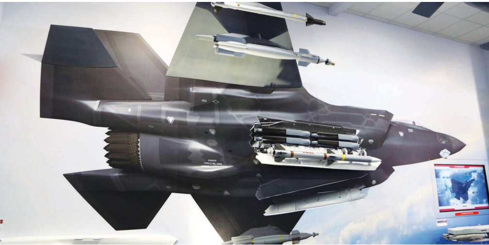
ASRAAM on external stores, Meteor and SPEAR missiles in F-35B weapons bay
