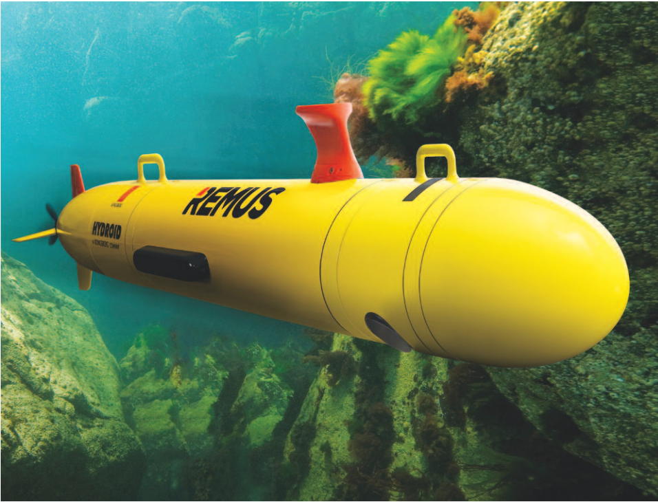
In the HA/DR mission, REMUS 100 AUVs equipped with bathymetry sensors and side scan sonars collected data on water depths and hazards to navigation, clear transit routes and anchorages for support vessels, data that fed into tactical recommendation products. Photo: Kongsberg
